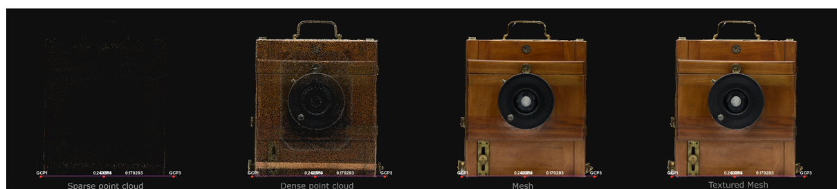
Fig. 3: From Sparse Point Cloud to Textured Mesh in 3DF Zephyr data processing.
